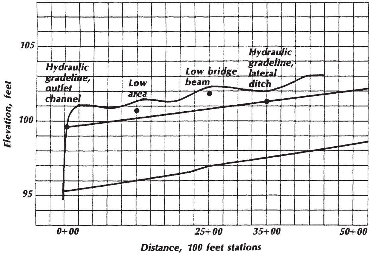
**Entrance of a subsurface drain into an outlet channel.**
