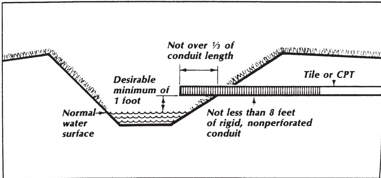
**Drawing A shows a lateral ditch graded through a spoil bank to discharge directly into an outlet channel.
