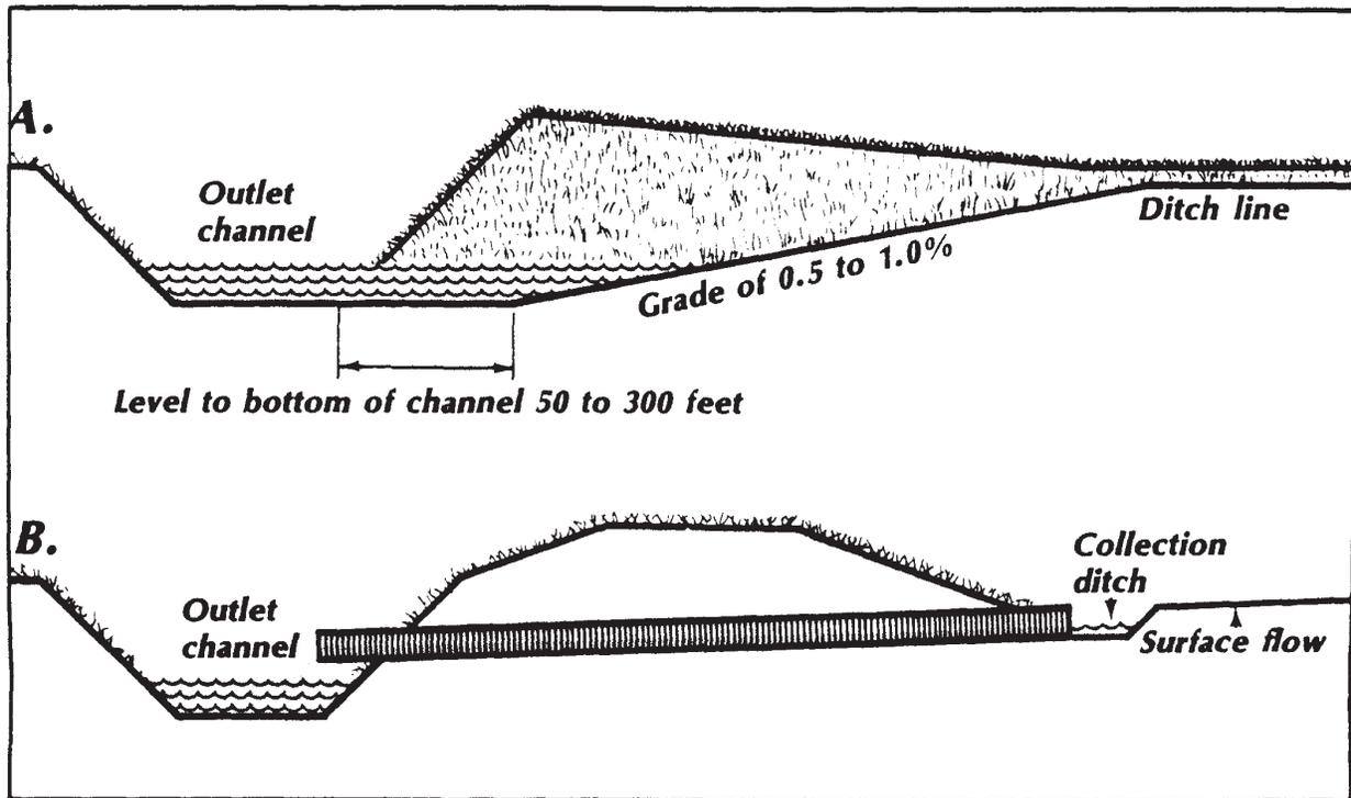
**Basic patterns for subsurface drainage systems (the arrows indicate the direction of water flow).**
