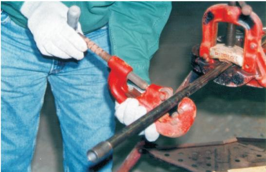
Using a wheel type pipe cutter.
