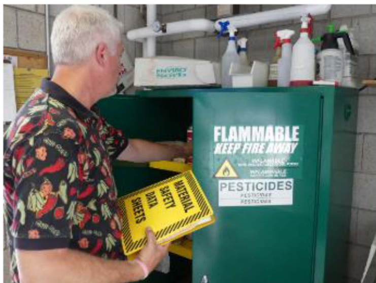
FIGURE 9.9 Chemicals such as pesticides should have their own locking storage cabinet that is designed to store them properly.
